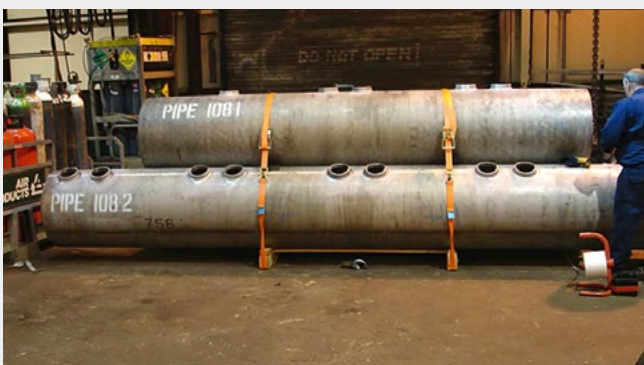
Extruded Manifolds Material : Alloy 800 HT
