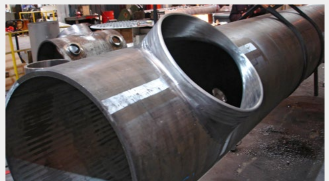
Extruded Manifolds Material : Alloy 800 HT
