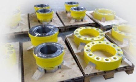
Swivel flanges to match API6A/API17D: 1 13/16" – 4 1/16" – 11" – 13 5/8" API 5K & API 10K Material: ASTM A694 F65 + A625 weld overlay Customer: SUBSEA 7
