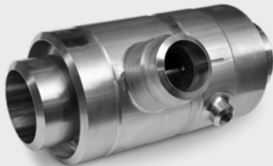
Special Double Tee for Pipe in Pipe Line: 8"x2"x3/4" Material: ASTM A694 F65 + A625 weld overlay Customer: TECHNIP
