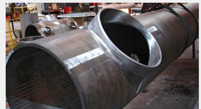
Extruded Manifolds Material : Alloy 800 HT
